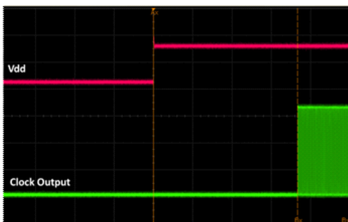
Figure 17. Startup Waveform vs. Vdd
