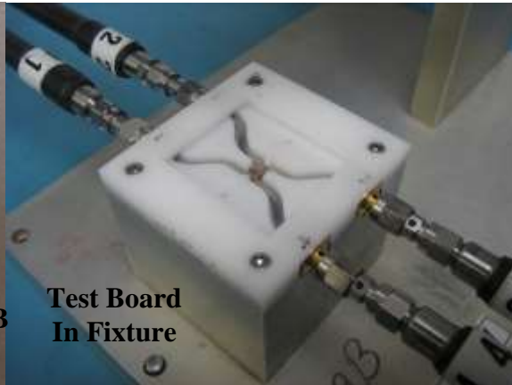
2dB, 3 dB and 5dB Test Board
