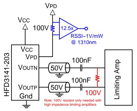
Optional RSSI implementation is shown in blue. Optional 100Ω differential termination for high impedance limiting amplifiers is shown in red.
