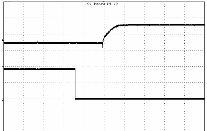
Figure 32: Turn on with Prebias 12Vin, 5V/0A out, Vbias = -3.3Vdc Top: 2V/div, 2ms/div, Bottom: 5V/div, 2ms/div
