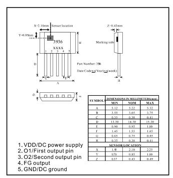
The PT3936 is designed for magnetic actuating using a bipolar magnetic field. The built-in dynamic offset cancellation of pre-amplifier stage achieves optimal symmetrical magnetic sensing. The output driver provides a linear drive to eliminate switching noise. This motor driver IC is especially designed for OA cooling fan solution or industry equipments such as inverters or fan trays.PT3936 provides FG function for users to monitor revolution. The supply voltage range is from 4.5V to 30V.
