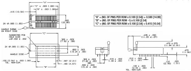
**ALL DIMENSIONS: INCHES [MILLIMETERS]** ALL TOLERANCES: ±0.005 [0.13] UNLESS OTHERWISE SPECIFIED DO NOT USE THIS SOCKET IN A BURN-IN OVEN WITH CONTACTS IN OPEN POSITION, AS IT WILL DAMAGE THE SOCKET CONSULT FACTORY FOR OTHER SIZES AND CONFIGURATIONS
