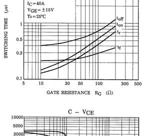
$\begin{array}{l} \text{COMMON EMITTER} \\ V_{\text{CC}} \! = \! 600 \text{V} \end{array}$
