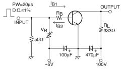
20I<sub>B1</sub>=-20I<sub>B2</sub>=I<sub>C</sub>=300mA (For PNP, the polarity is reversed.)
