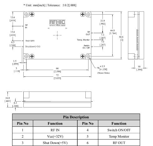
\* Recommended Screw Torque : 8.0kgf.cm±1 using SEMS M3 14mm Bolt
