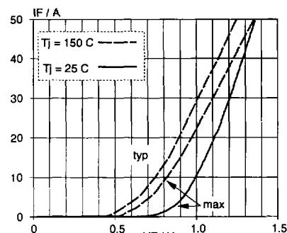
*Fig.9. Typical and maximum forward characteristic
