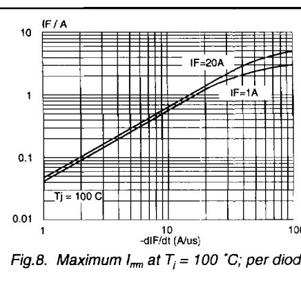
Fig.8. Maximum  $I_{mm}$  at  $T_j = 100^\circ C$ ; per diode
