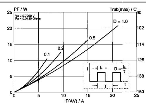
Fig.3. Maximum forward dissipation  $P_F = f(IF_{AV})$  per diode; square current waveform where  $I_{F(RMS)} = I_{F(AV)} \times \sqrt{D}$ .
