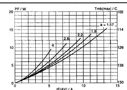
Fig.4. Maximum forward dissipation  $P_F = f(IF_{AV})$  per diode; sinusoidal current waveform where  $a$  = form factor =  $I_{F(RMS)} / I_{F(AV)}$ .
