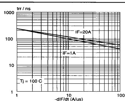
Fig.6. Maximum  $t_{rr}$  at  $T_j = 100^\circ C$ ; per diode
