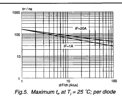
Fig.5. Maximum  $t_{rr}$  at  $T_j = 25^\circ C$ ; per diode
