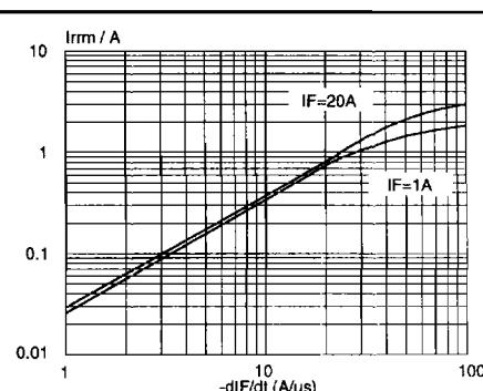
Fig.7. Maximum  $I_{mm}$  at  $T_j = 25^\circ C$ ; per diode
