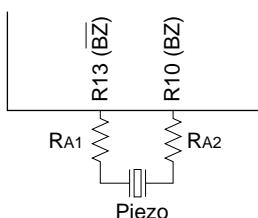
When the piezoelectric buzzer is driven directly
