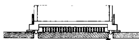
Tab for positioning on the PC board. Suitable for both manual and automatic insertion.
