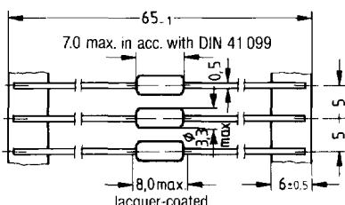
Smallest possible lead spacing 10 mm
