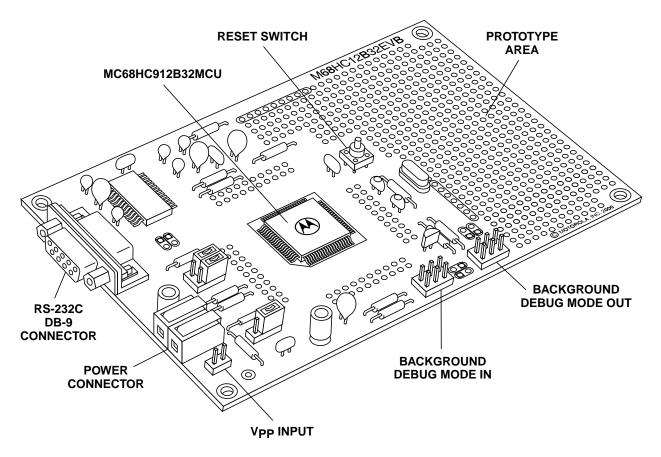
Figure 1. Evaluation Board Layout
