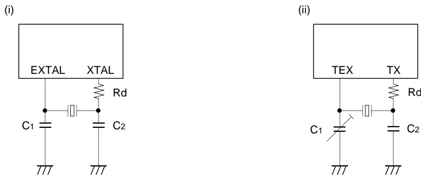
Fig. 13. Recommended oscillation circuit
