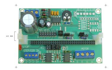
INFO The baseboard BB-035 allows to build a ready to use stepper driver unit using the TMCM-035 driver module. All important signal and power lines are accessible via screw terminals, the step and direction inputs are equipped with opto couplers. The integrated switch-mode regulator provides the required 5V supply voltage for the TMCM-035.
