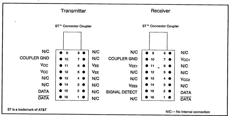
Pin 10 on both the transmitter and receiver is internally connected to the metal ST™ connector coupler. Depending on application, Pin 10 should be connected to chassis or circuit ground. The data links are designed to withstand a 15 kV pulse
