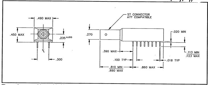
The package provides molded-in standoffs to allow for proper cleaning beneath the part after soldering. Parts are shipped with a plastic cap to protect the optical interface during attachment to the printed circuit boards.
