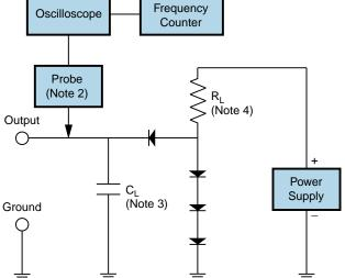
Note 1: An external 0.1µF low frequency tantalum bypass capacitor in parallel with a 0.01µF high frequency ceramic bypass capacitor close to the package ground and V<sub>DD</sub> pin is required.
