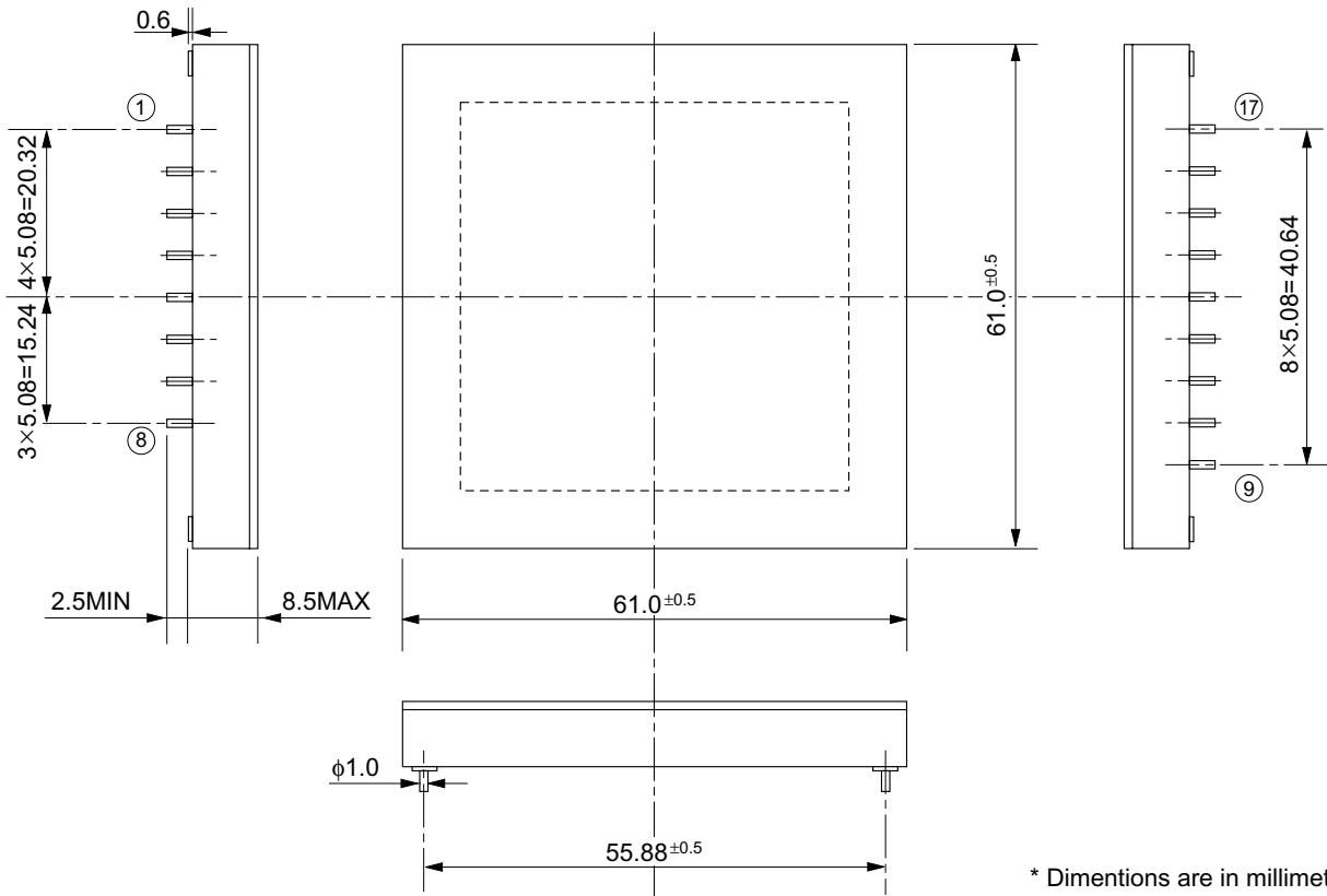
\* Dimensions are in millimeters.
