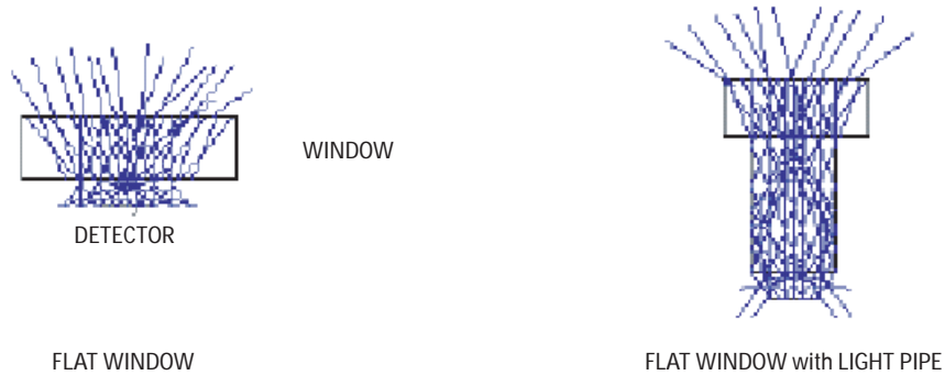
Figure 12. Recommended window design.
