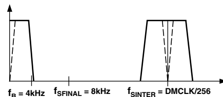
d. Final Filter LPF (HPF) Transfer Function
