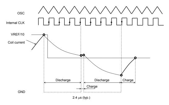
(4) Operation on change of predetermined current value (when in Charge mode)
