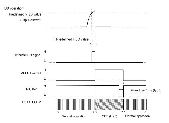
Note: The ISD circuit is activated if the absolute maximum current rating is violated. Note that the circuit is provided as an auxiliary only and does not necessarily provide the IC with a perfect protection from damages due to overcurrent caused by power fault, ground fault, load-short and the like.
