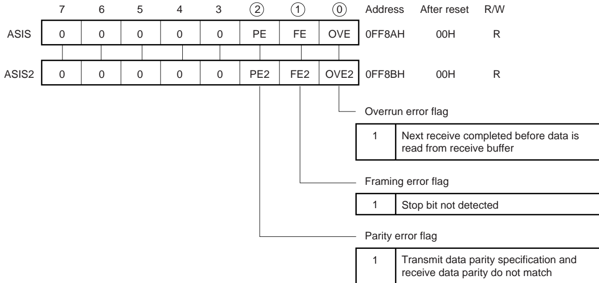
Figure 18-4. Format of Asynchronous Serial Interface Status Register (ASIS) and Asynchronous Serial Interface Status Register 2 (ASIS2)
