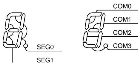
Figure 16-6 Example of COM, SEG Pin Connection (1/4 Duty)
