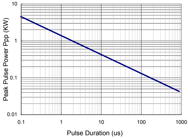
FIG 3 Admissible Power Dissipation Curve
