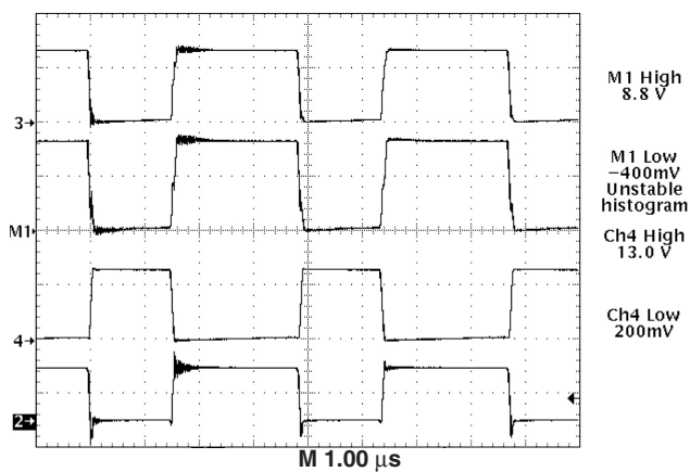
Trace 3 = V_{GATE(H)} (10 V/div.) Math 1 = V_{GATE(H)} - 5.0\text{ V}_{IN} Trace 4 = V_{GATE(L)} (10 V/div.) Trace 2= Inductor Switching Nodes (5.0 V/div.)
