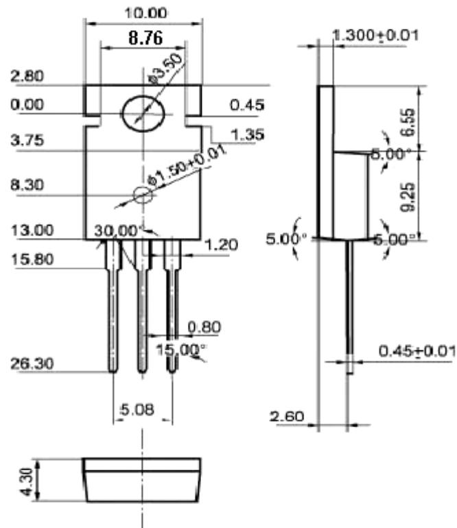
Fig.2 Outline dimensions (unindicated tolerance: 0.1mm)
