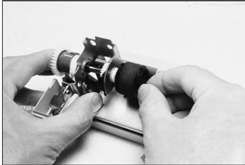
Figure 20 Replacing the Pickup Roller
