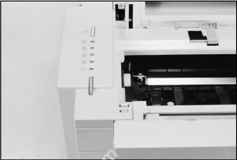
Figure 17 Left Side Cover Release Latch (5P/5MP shown)
