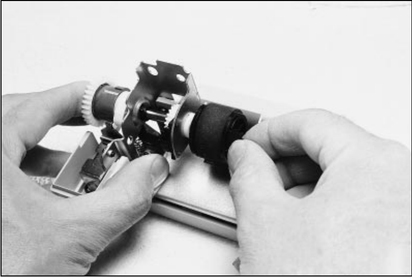
Figure 23 Replacing the Pickup Roller
