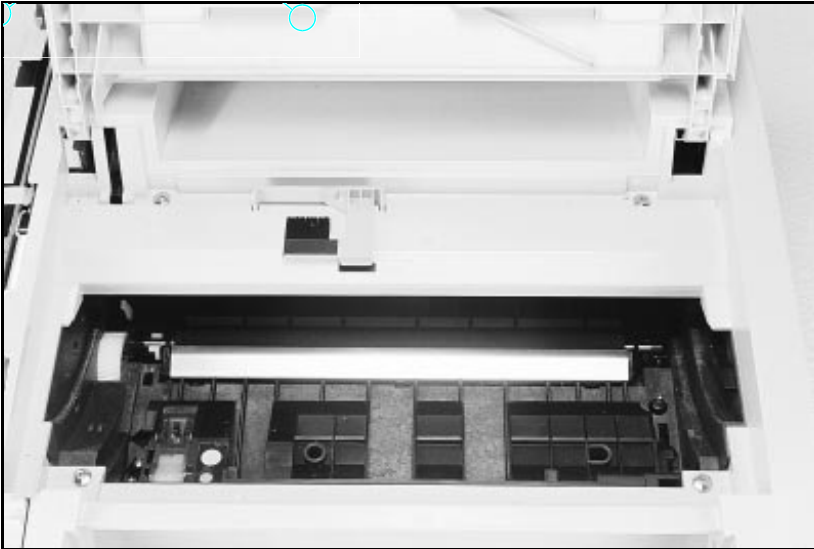
Figure 18 Removing the Top Cover Screws
