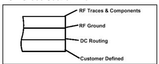
PCB dielectric between RF traces and RF ground layers should be chosen to reduce discontinuities between 50  $\Omega$  lines and package pins. M/A-COM recommends an FR-4 dielectric thickness of 0.008" (0.2 mm) yielding a 50  $\Omega$  line width of 0.015" (0.38 mm). The recommended metalization thickness is 1 oz. Copper.
