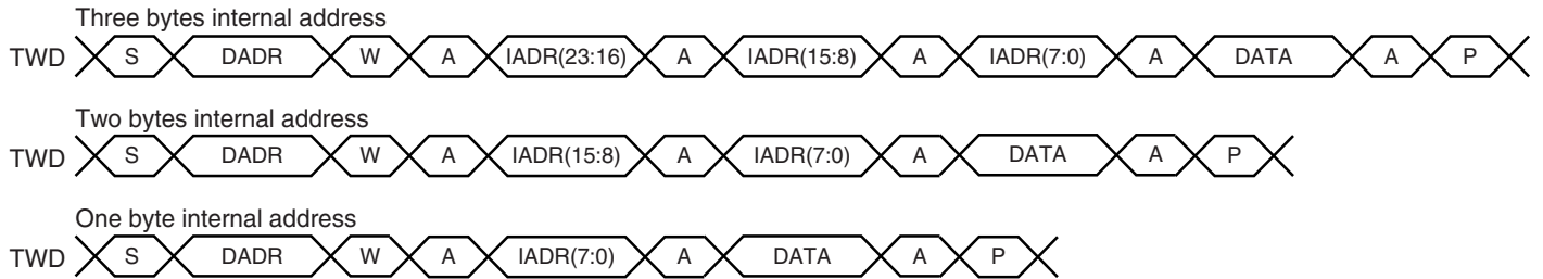
Figure 29-5. Master Write with One, Two or Three Bytes Internal Address and One Data Byte
