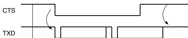
Figure 30-18. Transmitter Behavior when Operating with Hardware Handshaking
