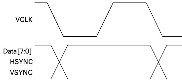
Data is asserted on the rising edge of VCLK (default) but can be programmed using the camera module registers to be asserted on the falling edge.
