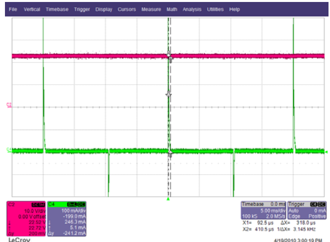
Figure 37 – 230 VAC, 5° Phase. Upper: V_{OUT} , 10 V / div. Lower: I_{IN} , 0.1 A / div., 5 ms / div.
