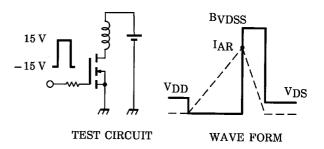
$$\begin{aligned} R_G &= 25~\Omega \\ V_{DD} &= 90~V,~L = 594~mH \end{aligned} \qquad EAS &= \frac{1}{2} \cdot L \cdot I^2 \cdot \left( \frac{BVDSS}{BVDSS - VDD} \right) \end{aligned}$$
