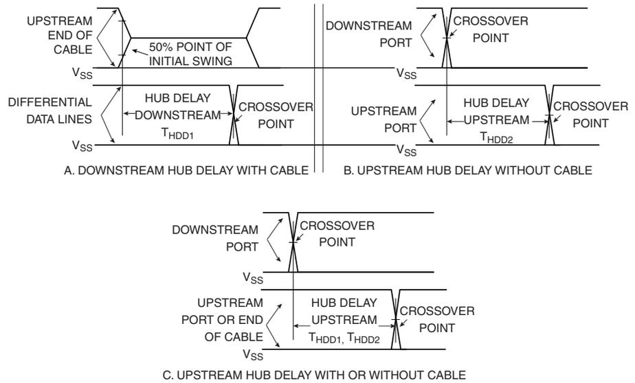
**Figure 12. Hub EOP Delay and EOP Skew**
