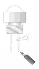
e) LEDs are static sensitive devices, so adequate handling precautions have to be taken, e.g. wearing grounding wrist straps.
