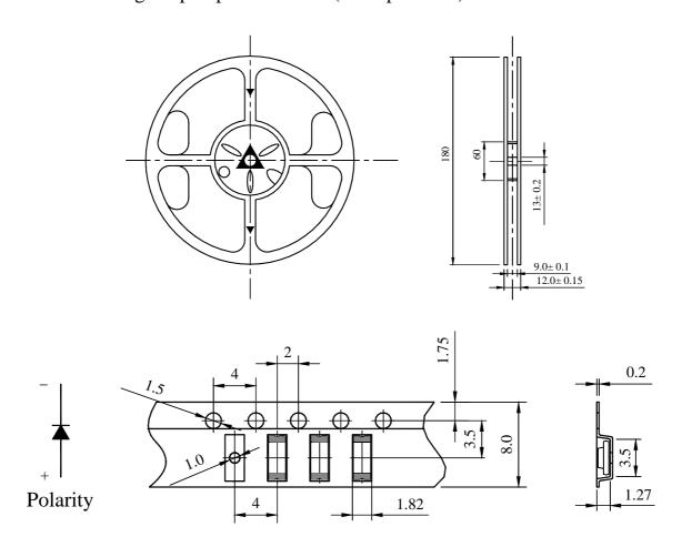
Reel Lead Min.60mm No LEDs
