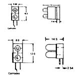
The colour combinations for these types are specified by replacing 'U' and 'L' with the letters R, G, Y or A (red, green, yellow or amber) to denote the Upper and Lower LED colours.
