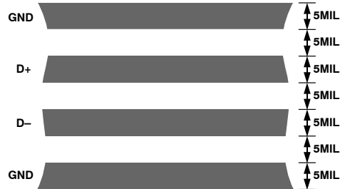
Figure 16. Arrangements of Signal Tracks
