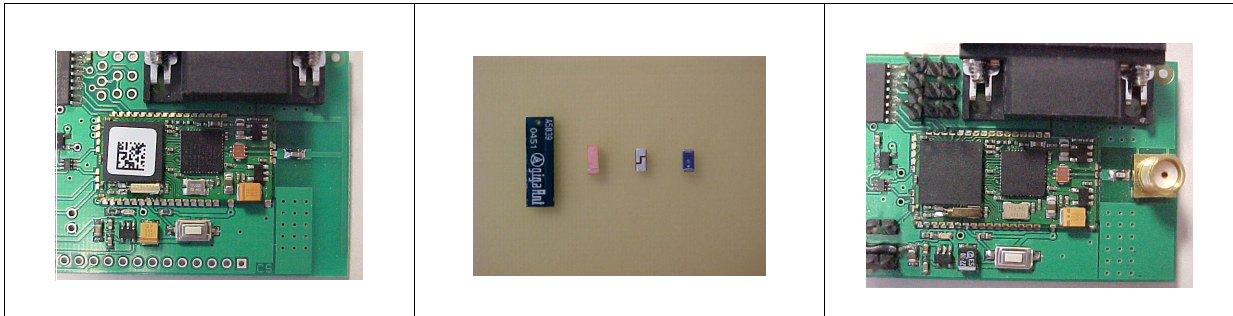
Figure 5. SMA connector for external antenna
