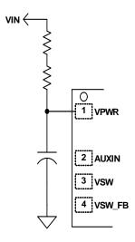
FIGURE 7. ADDING DROPPING RESISTORS TO VPWR
