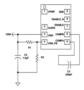
FIGURE 5. VSW ADJUSTMENT AND COMPENSATION
