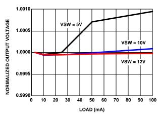
FIGURE 4. VSW REGULATION vs LOAD @ VPWR = 18V, AUXIN = 15V, +25°C
