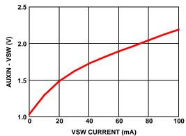
FIGURE 2. AUXIN - VSW vs I<sub>VSW</sub> @ VPWR = 17V, +25°C
