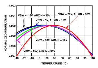
FIGURE 3. VSW REGULATION vs TEMPERATURE @ VPWR = 100V, I<sub>VSW</sub> = 3mA
