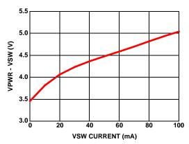
FIGURE 1. VPWR - VSW vs I<sub>VSW</sub> @ AUXIN = 0V, +25°C
