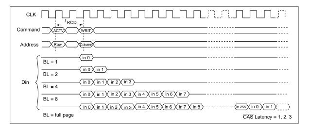
**Single write:** A single write operation is enabled by setting OPCODE (A9, A8) to (1, 0). In a single write operation, data is only written to the column address (AY0 to AY8; HM5216805 Series, AY0 to AY9; HM5216405 Series) and the bank select address (A11) specified by the write command set cycle without regard to the burst length setting. (The latency of data input is 0).
