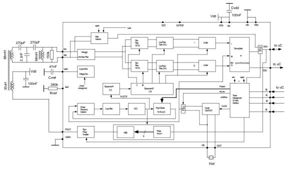
Note: pins TEST and SUPTEST remain unconnected
