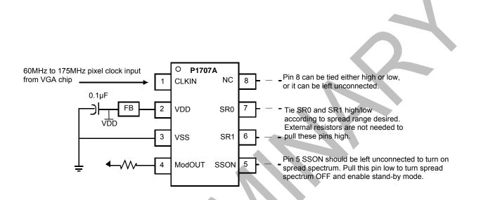
Note: To set the P1707A to standby mode, disable the input clock (pin 1 CLKIN) and pull SSON (pin 5) low. *Refer Standby Mode Selection Table.*
