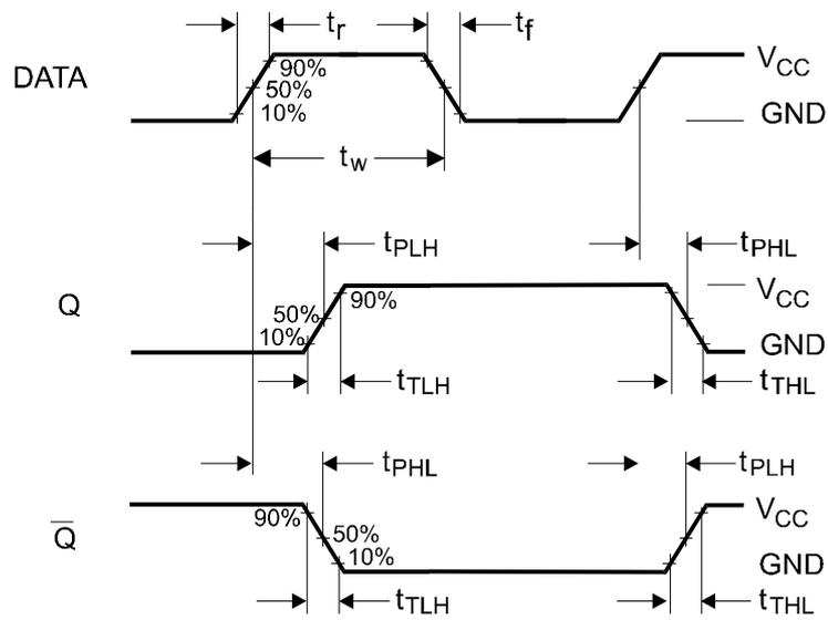
Figure 2. Switching Waveforms
