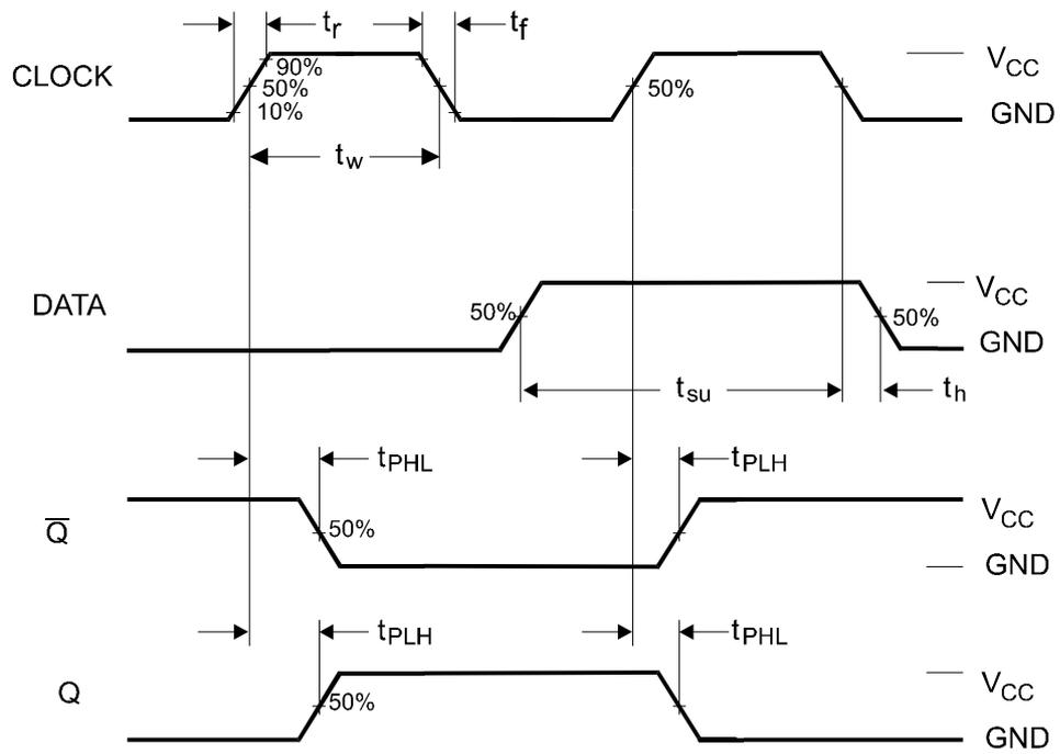
Figure 1. Switching Waveforms
