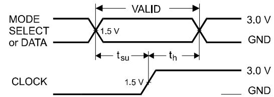
**Figure 4. Switching Waveform**
