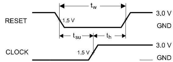
**Figure 2. Switching Waveform**
