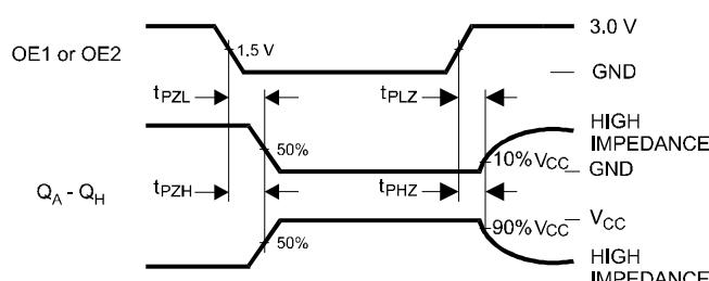
**Figure 3. Switching Waveform**
