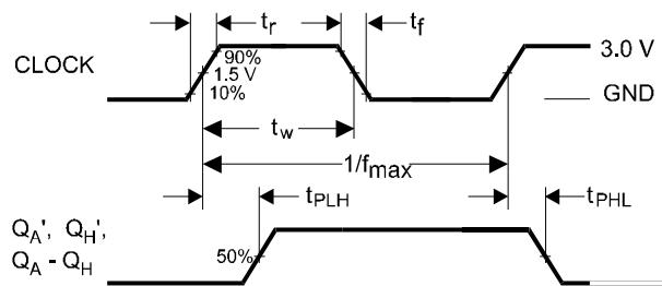
**Figure 1. Switching Waveform**
