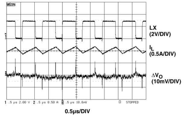
FIGURE 16. PWM STEADY-STATE OPERATION ( $I_O = 1A$ )
