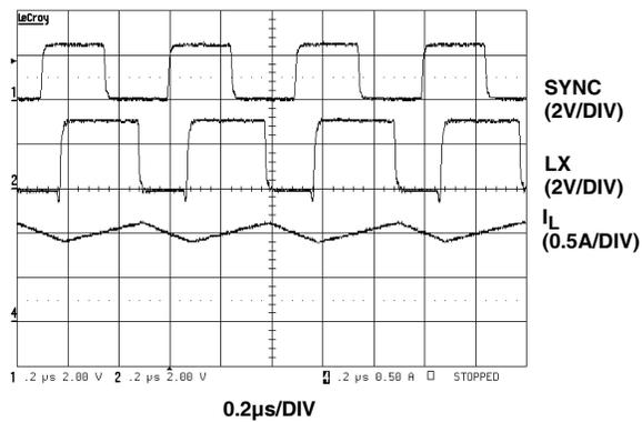
FIGURE 17. EXTERNAL SYNCHRONIZATION TO 2MHz
