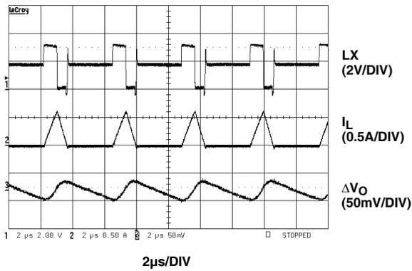
FIGURE 15. PFM STEADY-STATE OPERATION WAVEFORM ( $I_O = 100mA$ )
