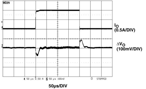
FIGURE 20. PWM LOAD TRANSIENT RESPONSE (0A TO 1A)
