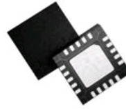
4mm x 4mm QFN Package
