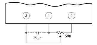
Adjust/comp (pin 3) may be driven by external circuitry referenced to pin 2 (-output) if desired. Grounding pin 3 causes voltage to increase (25% typically) while driving pin 3 above 1.3V causes output voltage to decrease. Pin 3 may be driven through  $10K\Omega$  or more if connection of the comp function is also required.
