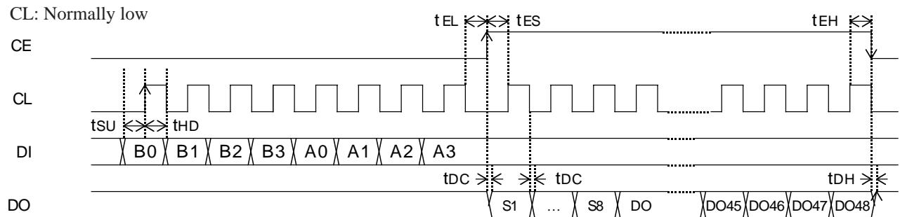
Note: Since the DO pin is an n-channel open-drain output, the data transition times ( $t_{DC}$  and  $t_{DH}$ ) differ depending on the value of the pull-up resistor used.
