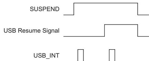
The device with remote wake up function can wake-up the USB Host by sending a wake-up pulse through RMWK (bit 1 of USC). Once the USB Host receive the wake-up signal from HT82K96E. it will send a Resume signal to device. The timing as follow:
