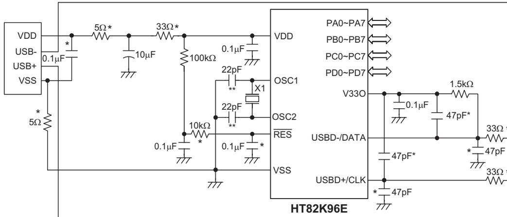
Note: The resistance and capacitance for reset circuit should be designed in such a way as to ensure that the VDD is stable and remains within a valid operating voltage range before bringing RES to high.
